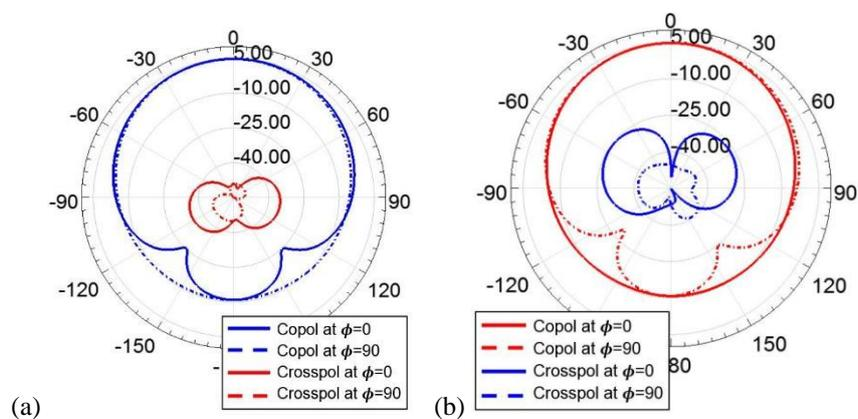
Fig. 3. Radiation Pattern for (a) H-Polarization and (b) V-Polarization.
