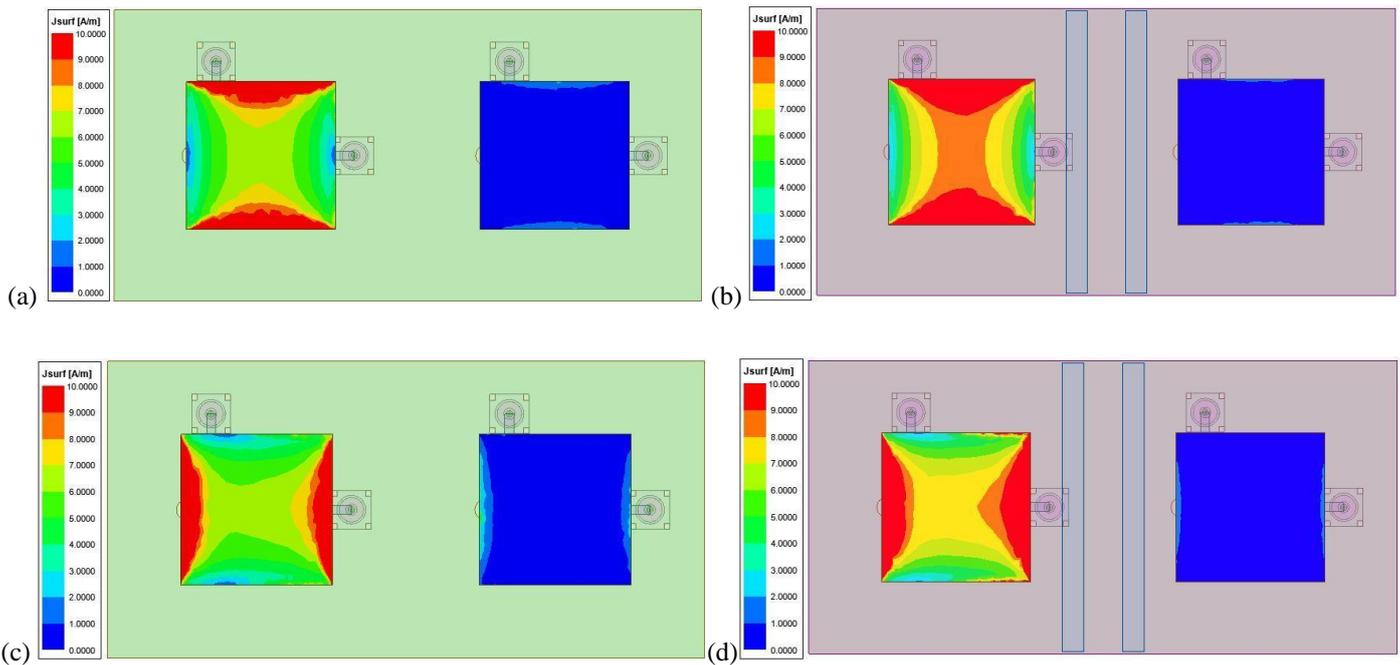
Fig. 6. Surface current plots (a) Normal 1X2 array and (b) 1X2 array with micro-striplines when H-port is excited (c) Normal 1X2 array and (d) 1X2 array with micro-striplines when V-port is excited.
