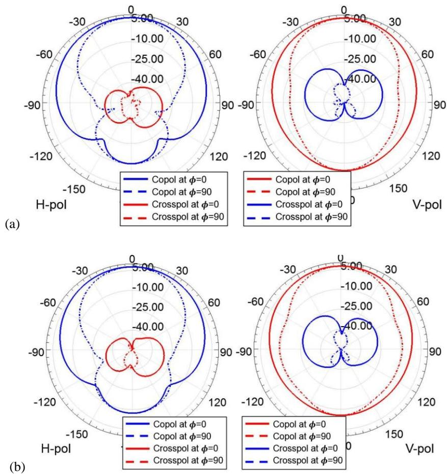
Fig. 7. Radiation patterns for 1X2 array (a) without striplines and (b) with striplines.
