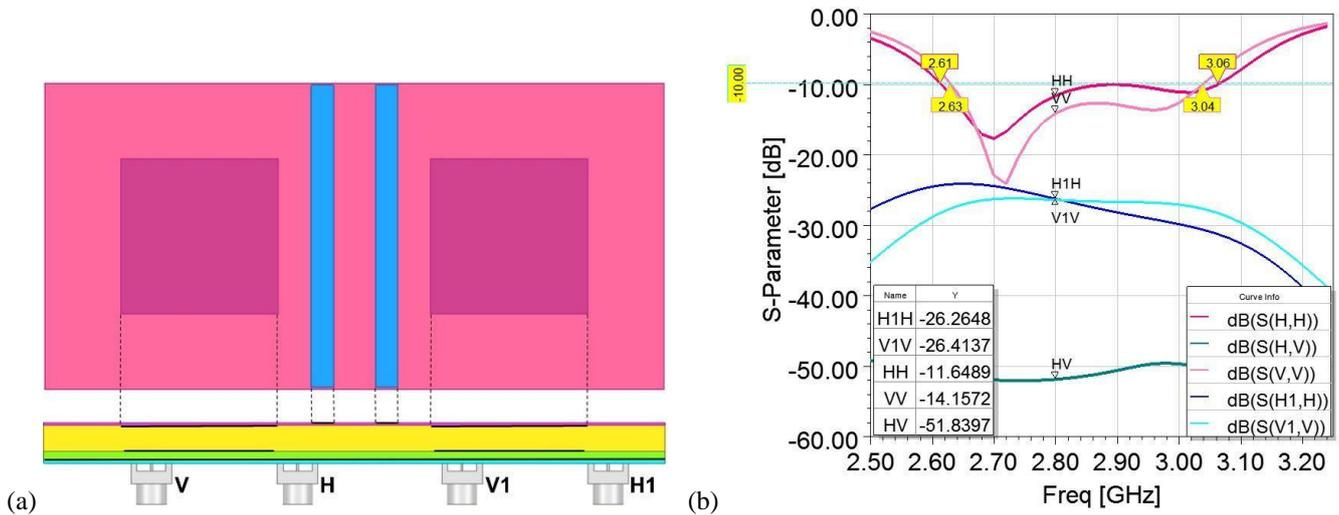
Fig. 5. (a) Top and side view of 2X1 array with striplines and (b) its S-Parameter plot.
