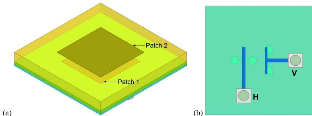
Fig. 1. Antenna Structure for (a) Isometric view and (b) Bottom view.
