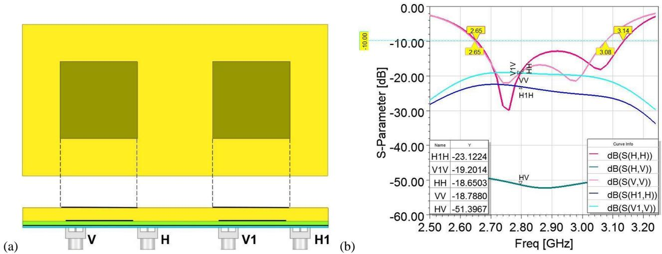
Fig. 4. (a) Top and side view of normal 2X1 array and (b) its S-Parameter plot.
